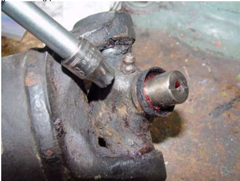
Cross shown with end caps removed. Remove the grease fitting
