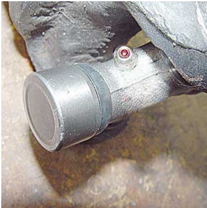
Do not put the last 2 end caps on yet. Reinstall the drive shaft. I was doing the rear which meant that I had to slip the yoke back into the output side of the transercase. It took some massaging with a pry bar to get the shaft lined up and pushed into the transercase.
