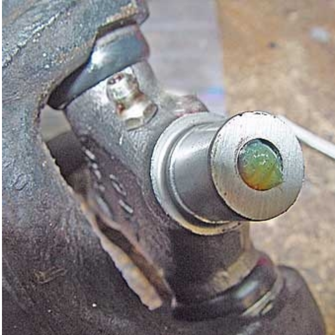
This shows the snap ring groove and snap ring. Shown is the cross with the end cap removed showing the grease path within the joint.
